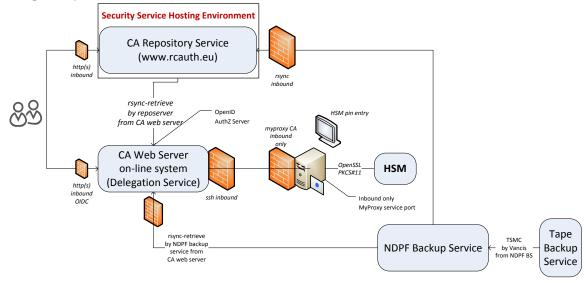
The CA web server on-line system ("Delegation Service") accepts connections on port http (80/tcp) and https (443/tcp) from the internet, serving both the web interface and user authentication consent and where-are-you-from-service and SAML and OpenID Connect protocol flows. It also accepts inbound rsync connections over a trusted network from the back-up service, inbound SSH connections from DCA Service management networks (not shown),
