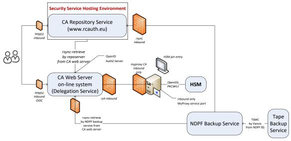
The hardware cryptographic module (HSM) is connected to the signing system through a USB port. The HSM interface software process on the signing machine uses the PIN of the HSM – provided in real-time by the CA operator – to activate the HSM over its encrypted USB connection, following which PKCS#11 requests can be sent to it.
